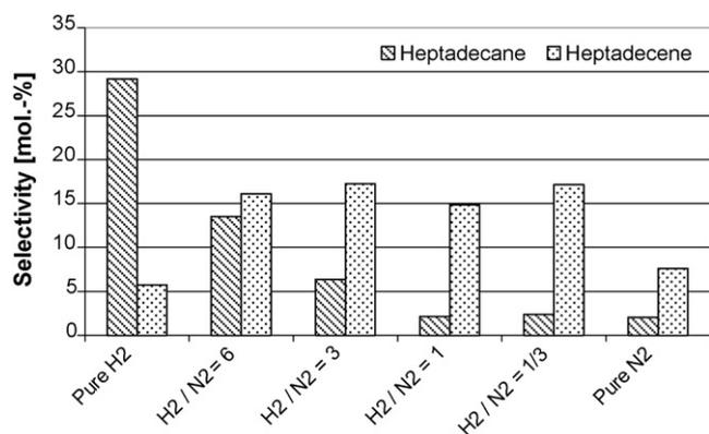
**Fig. 9.** Heptadecane vs heptadecene selectivity depending on hydrogen:nitrogen ratio; reaction conditions:  $T = 380^\circ\text{C}$ ,  $\dot{V}_{\text{total}} = 50\text{ ml/min}$ ,  $\dot{m}_{\text{OA}} = 6.2\text{ ml/h}$ ,  $m_{\text{Catalyst}} = 3\text{ g}$ .
