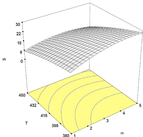
**Fig. 6.** C17 selectivity ( $S$  in mol%) plotted over reaction temperature ( $T$  in °C) and catalyst mass ( $m$  in g),  $\dot{V}_{H_2} = 50$  ml/min,  $\dot{m}_{OA} = 6.2$  ml/h.
