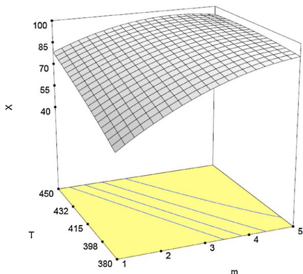
**Fig. 5.** Conversion ( $X$  in mol%) plotted over reaction temperature ( $T$  in °C) and catalyst mass ( $m$  in g),  $\dot{V}_{H_2} = 50$  ml/min,  $\dot{m}_{OA} = 6.2$  ml/h.
