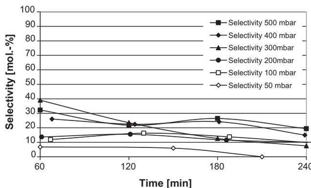
**Fig. 8.** C17 selectivity at different absolute pressures over time on stream; reaction conditions:  $T = 350$  °C,  $\dot{V}_{H_2} = 50$  ml/min,  $\dot{m}_{OA} = 6.2$  ml/h,  $m_{Catalyst} = 3$  g.
