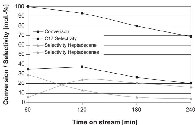
**Fig. 3.** Conversion and C17 selectivity of a reference reaction plotted over time on stream; C17 selectivity is the combination of the selectivities to heptadecane and all heptadecene isomers (grey lines); reaction conditions:  $T = 380\text{ }^{\circ}\text{C}$ ,  $V_{\text{H}_2} = 50\text{ ml/min}$ ,  $m_{\text{OA}} = 6.2\text{ ml/h}$ ,  $m_{\text{catalyst}} = 3\text{ g}$ .
