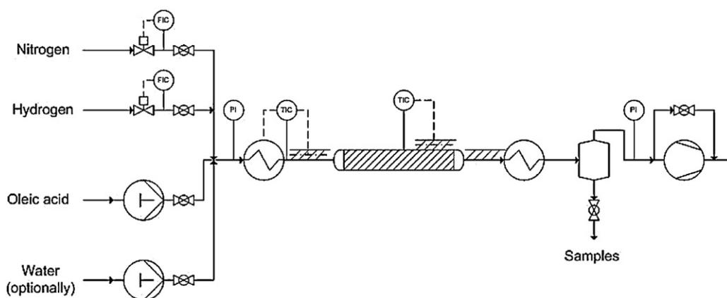
Fig. 1. Schematic reactor setup.
