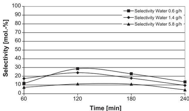
**Fig. 11.** C17 selectivity plotted over time on stream with varying water mass flows; reaction conditions:  $T = 380^\circ\text{C}$ ,  $\dot{V}_{\text{H}_2} = 50\text{ ml/min}$ ,  $\dot{m}_{\text{OA}} = 6.2\text{ ml/h}$ ,  $m_{\text{Catalyst}} = 3\text{ g}$ .
