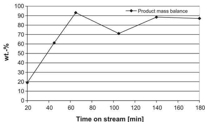
**Fig. 4.** Mass balance of all collected liquid products over time on stream; reaction conditions:  $T = 380\text{ }^{\circ}\text{C}$ ,  $V_{\text{H}_2} = 50\text{ ml/min}$ ,  $m_{\text{OA}} = 6.2\text{ ml/h}$ ,  $m_{\text{catalyst}} = 5\text{ g}$ .
