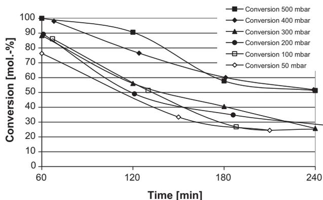
**Fig. 7.** Conversion at different absolute pressures over time on stream; reaction conditions:  $T = 350$  °C,  $\dot{V}_{H_2} = 50$  ml/min,  $\dot{m}_{OA} = 6.2$  ml/h,  $m_{Catalyst} = 3$  g.
