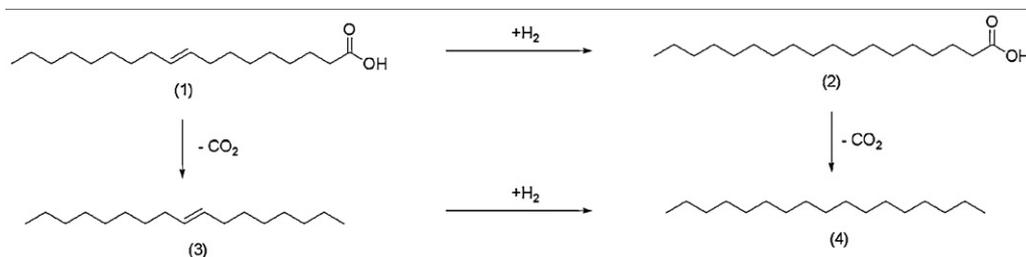
Fig. 2. Reaction scheme: deoxygenation of oleic acid.
