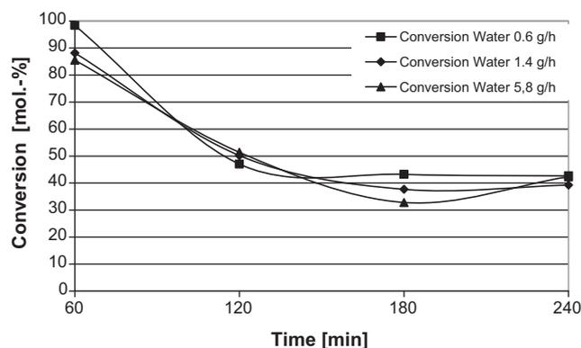
**Fig. 10.** Conversion plotted over time on stream with varying water mass flows; reaction conditions:  $T = 380^\circ\text{C}$ ,  $\dot{V}_{\text{H}_2} = 50\text{ ml/min}$ ,  $\dot{m}_{\text{OA}} = 6.2\text{ ml/h}$ ,  $m_{\text{Catalyst}} = 3\text{ g}$ .
