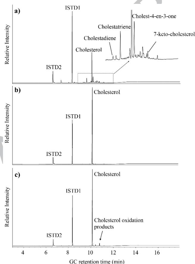
**Figure 1.** GC-FID chromatograms of cholesterol and cholesterol oxidation products extracted from experiments 1 (a), 4 (b) and 3 (c). The internal standards (ISTD1 and ISTD2) are at the same concentrations in all three chromatograms. The magnified section of chromatogram in panel a) shows the cholesterol oxidation products eluting between 9 and 12 min (identified by GC-MS).
