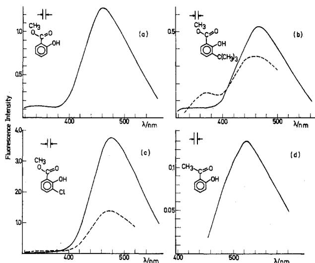
**Figure 1.** Corrected emission spectra on the same intensity scale (see text): (a)  $10^{-5}$  M methylsalicylate in cyclohexane; (b) methyl 3-*tert*-butylsalicylate and (c) methyl 3-chlorosalicylate, both  $10^{-5}$  M, in cyclohexane (—) and ethanol (---); (d)  $10^{-5}$  M *o*-hydroxyacetophenone in cyclohexane. The excitation wavelength was 290 nm for (a), (b), and (c), and 320 nm for (d).
