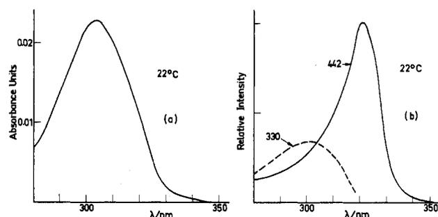
**Figure 2.** Absorption (a) and corrected fluorescence excitation spectra (b) including wavelength sensitivity factors (see text) or methylsalicylate in gas phase at equilibrium pressure, for the indicated emission wavelengths and temperature. The excitation slit was 1 nm.
