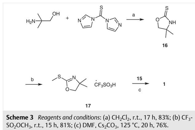
**Scheme 3** Reagents and conditions: (a) CH<sub>2</sub>Cl<sub>2</sub>, r.t., 17 h, 83%; (b) CF<sub>3</sub>SO<sub>2</sub>OCH<sub>3</sub>, r.t., 15 h, 81%; (c) DMF, Cs<sub>2</sub>CO<sub>3</sub>, 125 °C, 20 h, 76%.
