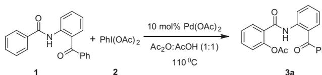
Scheme 1. Acetoxylation of *N*-(2-benzoylphenyl)benzamide.
