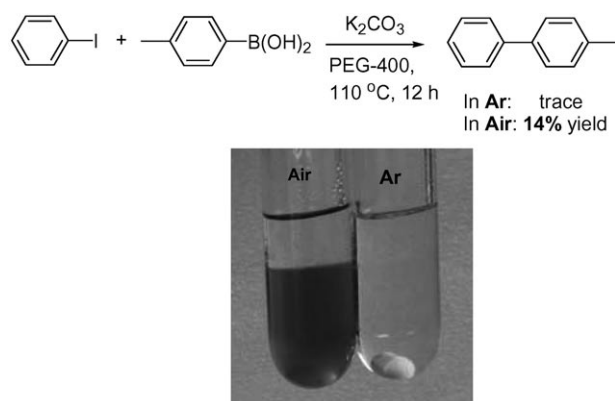
Figure 1. The different colours between the catalytic reaction performed in air or argon atmosphere (the reaction was quenched with 2 mL of water and 2 mL of ethyl acetate).
