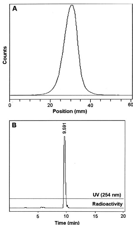
Fig. 2. (A) Radio thin-layer chromatogram of radioiodine-labeled PETG. Developing solvents: 19:1  $\text{CH}_3\text{CN}-\text{H}_2\text{O}$ ;  $R_f$  0.66; (B) HPLC analysis. HPLC conditions: 7:3  $\text{H}_2\text{O}-\text{CH}_3\text{CN}$ ; flow rate, 1.0 mL/min;  $t_R$  9.59 min. The eluant was simultaneously monitored by a UV detector (254 nm) and a NaI(Tl) radioactivity detector.
