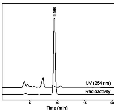
Fig. 1. HPLC profile of 1,3,4,6-tetraacetyl 4- $^{123}\text{I}/^{125}\text{I}$ iodo-PETG. HPLC conditions: 80:19:1 *n*-hexanes- $\text{CH}_2\text{Cl}_2$ -2-propanol; flow rate, 4.0 mL/min;  $t_R$  9.57 min. The eluant was simultaneously monitored by a UV detector (254 nm) and a NaI(Tl) radioactivity detector.
