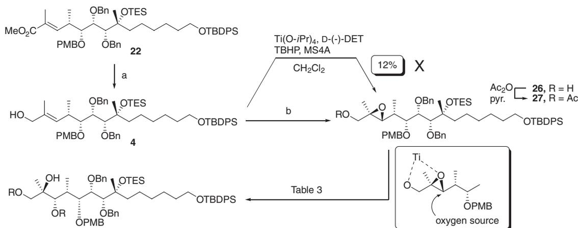
Scheme 8. Asymmetric epoxidation of **4** (route B); Reagents and conditions: (a)  $\text{LiBH}_4$ , THF (100%). (b) *m*CPBA,  $\text{NaHCO}_3$ ,  $\text{CH}_2\text{Cl}_2$  (75%).
