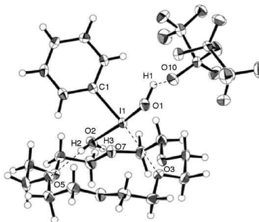
Figure 2. ORTEP drawing of **8**-[18]C6 with thermal ellipsoids drawn at the 50% probability level. Selected bond lengths [Å] and angles [°]: I1–C1 2.106(6), I1–O1 1.955(5), I1–O2 2.381(5), I1–O3 2.893(4), O10...H1 1.819, O5...H2 1.968, O7...H3 1.810; C1–I1–O1 92.8(2), C1–I1–O2 82.00(18), O1–I1–O2 174.43(16).
