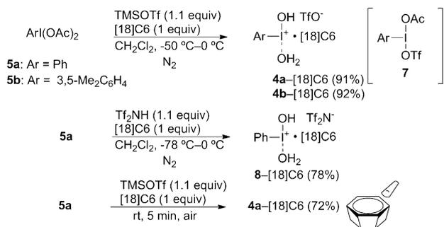
Scheme 4. Synthesis of aquo(hydroxy)- $\lambda^3$ -iodane-[18]C6 complexes.
