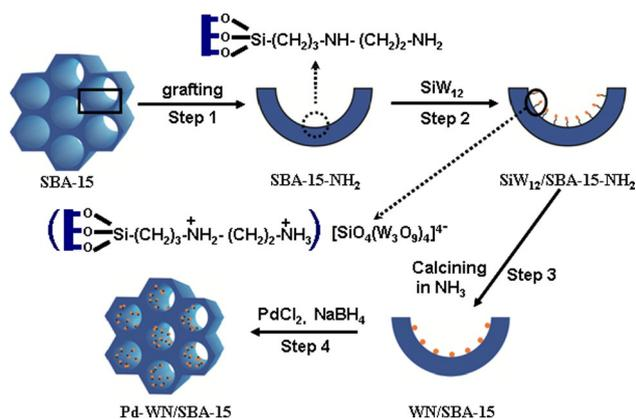
**Scheme 2.** Synthetic scheme for the construction of the ternary Pd-WN/SBA-15 catalyst.
