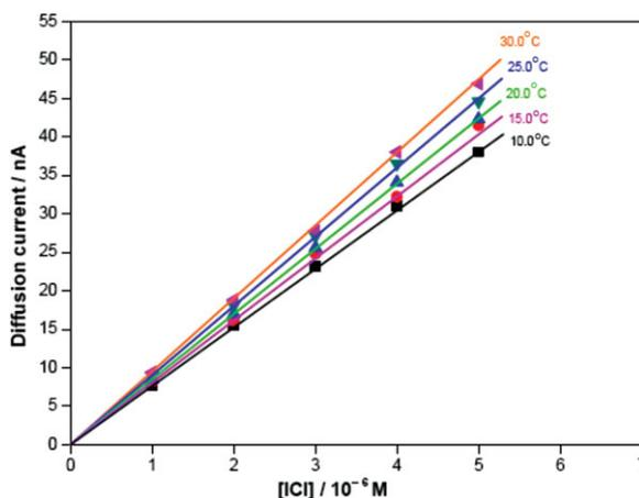
**Figure 1** Calibration of the diffusion current of ICl at various temperatures for the uncatalyzed iodination of phenol in aqueous medium at pH 4.8.
