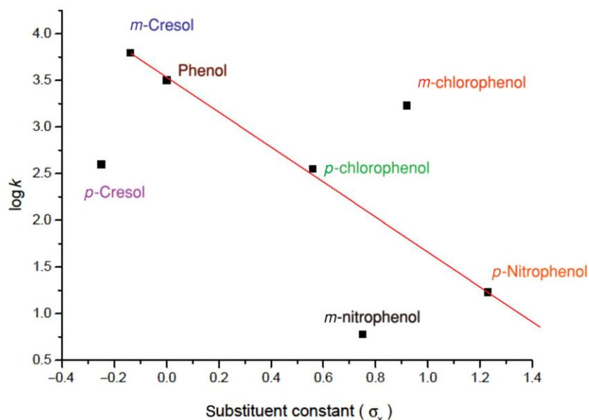
Figure 4 Hammett plot for the iodination reactions studied.
