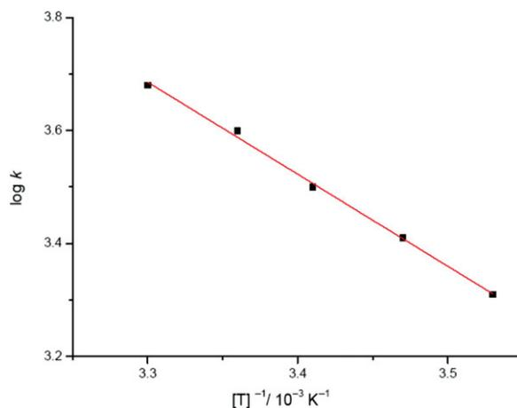
**Figure 3** Variation of the specific reaction rate of iodination of phenol by ICl in aqueous medium at different temperatures at pH 4.8.
