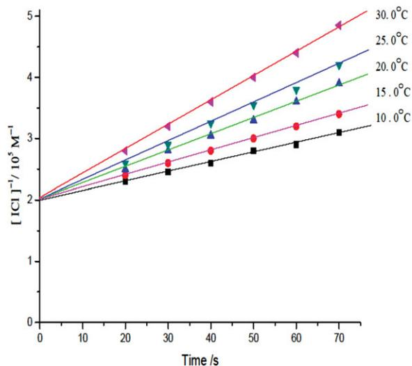
**Figure 2** Kinetics of the uncatalyzed iodination of phenol by ICl in aqueous medium at various temperatures at pH 4.8.
