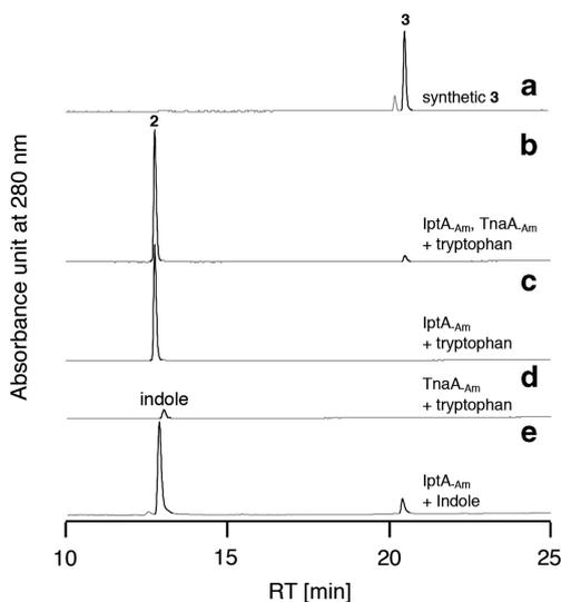
**Figure 4** UV chromatograms from the LC-MS analysis of the products of the *in vitro* enzyme reaction using recombinant IptA<sub>Am</sub> and TnaA<sub>Am</sub>. (a) Synthetic standard of 6-DMAI (3). (b) 2 and 3 are produced from tryptophan in the presence of both IptA<sub>Am</sub> and TnaA<sub>Am</sub>. (c) 2 is produced from tryptophan by IptA<sub>Am</sub>. (d) Indole is produced from tryptophan by TnaA<sub>Am</sub>. (e) A trace amount of 6-DMAI is produced from indole by IptA<sub>Am</sub>.
