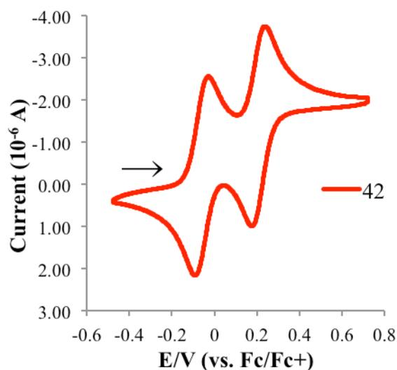
**Figure 8.** Cyclic voltammogram of **42**. Recorded in acetonitrile; 0.1 M electrolyte [*n*-Bu<sub>4</sub>N][ClO<sub>4</sub>];  $\nu = 100 \text{ mVs}^{-1}$ ; Pt working electrode, Ag/AgCl reference electrode and Pt counter electrode.
