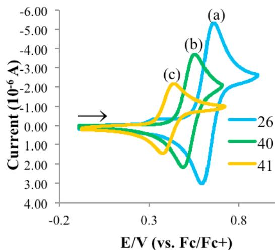
**Figure 7.** Cyclic voltammograms of (a) **26**, (b) **40** and (c) **41**. Recorded in acetonitrile; 0.1 M electrolyte [*n*-Bu<sub>4</sub>N][ClO<sub>4</sub>];  $\nu = 100 \text{ mVs}^{-1}$ ; Pt working electrode, Ag/AgCl reference electrode and Pt counter electrode.
