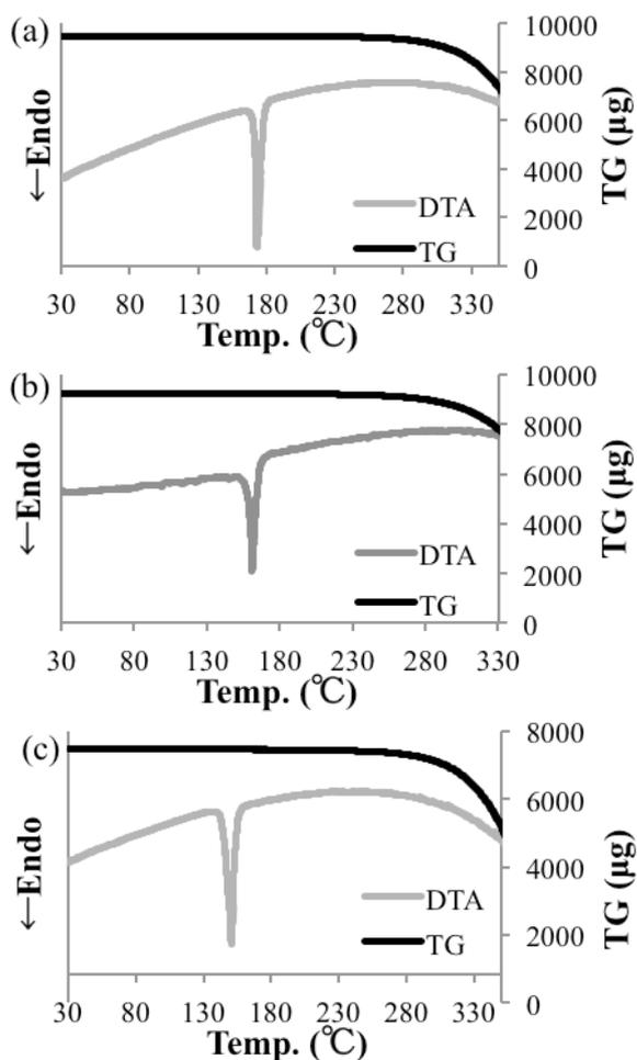
**Figure 10.** TG-DTA curve of (a) **26**, (b) **27** and (c) **31** at heating rate of 5 K min<sup>-1</sup> under N<sub>2</sub> atmosphere.
