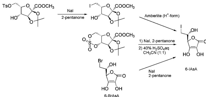
**Scheme 1.** Synthetic route for 6-deoxy-6-iodo-L-ascorbic acid (6-IAsA).
