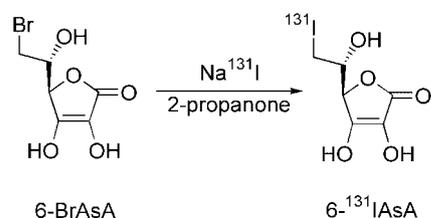
**Scheme 2.** Radiochemical synthesis of 6-deoxy-6- $^{131}\text{I}$ iodo-L-ascorbic acid (6- $^{131}\text{I}$ AsA) by exchange of radioiodine for bromide.
