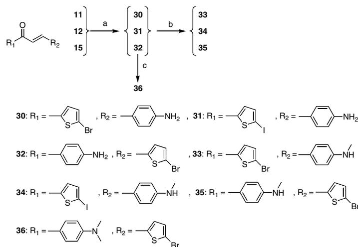
Scheme 3. Reagents: (a) EtOH, SnCl<sub>2</sub>; (b) CH<sub>3</sub>I, K<sub>2</sub>CO<sub>3</sub>, DMSO; (c) AcOH, (CH<sub>2</sub>O)<sub>n</sub>, NaCNBH<sub>3</sub>.
