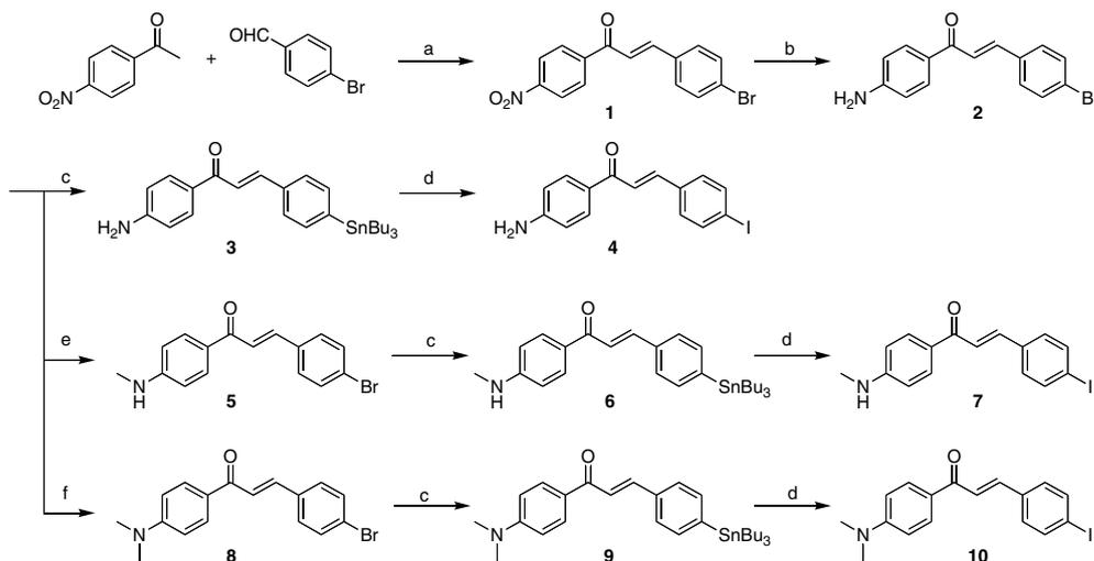
**Scheme 1.** Reagents: (a) EtOH, KOH; (b) EtOH, SnCl<sub>2</sub>; (c) dioxane, (Bu<sub>3</sub>Sn)<sub>2</sub>, (Ph<sub>3</sub>P)<sub>4</sub>Pd, Et<sub>3</sub>N; (d) CHCl<sub>3</sub>, I<sub>2</sub>; (e) CH<sub>3</sub>I, K<sub>2</sub>CO<sub>3</sub>, DMSO; (f) AcOH, (CH<sub>2</sub>O)<sub>m</sub>, NaCNBH<sub>3</sub>.
