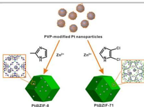
**Scheme 1.** The synthetic process of Pt NP embedded MOF composite catalysts and the crystallographic structures of corresponding ZIF-8 and ZIF-71 matrix.
