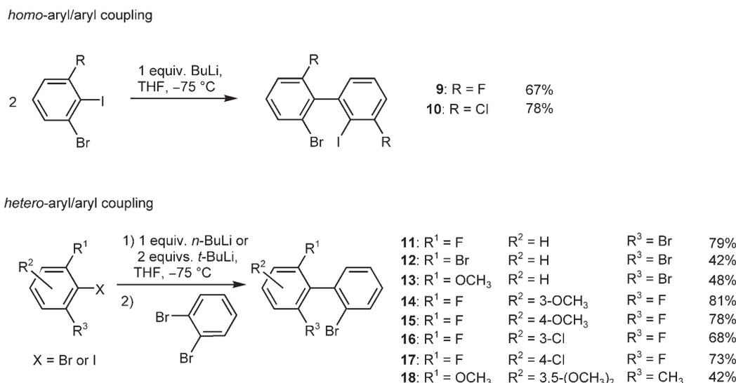
**Scheme 4.** Synthesis of *ortho,ortho'*-trisubstituted biaryls by *homo*- and *hetero*-aryl/aryl coupling.
