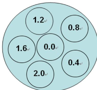
Fig. 1. Schematic drawing of a phantom assembled with six tubes consisting of a concentration series of Gd(III)-L or Gd(III)-DTPA solutions. Numbers indicated in tubes showed the concentrations of Gd(III)-L or Gd(III)-DTPA ( mM ). The center tube contained water only. The larger circle surrounding the six tubes is the outer tube, filled with 0.2 %  $\text{CuSO}_4$  solution. The six-tube phantom was immersed in the solution to reduce artifacts.
