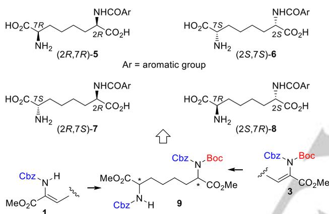
Figure 2. Synthetic plan for **5–8**.
