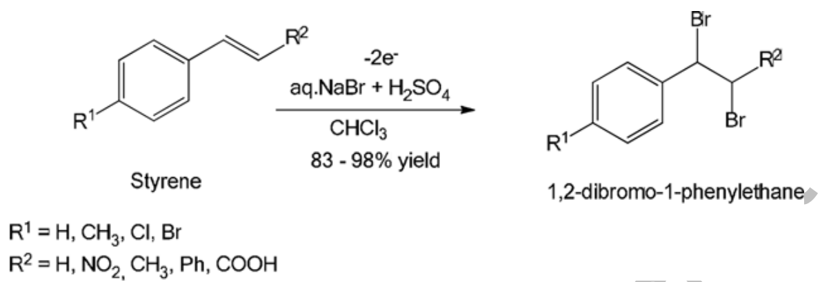
Figure 1. Scheme for electrochemical bromination of styrene
