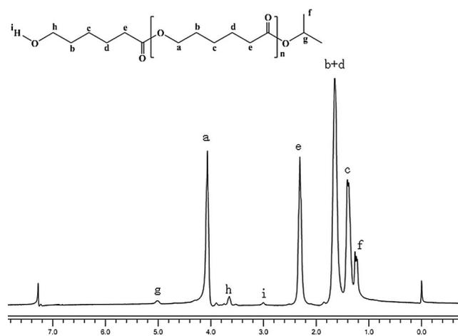
**Figure 4.** <sup>1</sup>H NMR spectrum of the oligomer of  $\epsilon$ -caprolactone initiated by complex **6**, and quenched by 2-propanol in  $\text{CDCl}_3$ .
