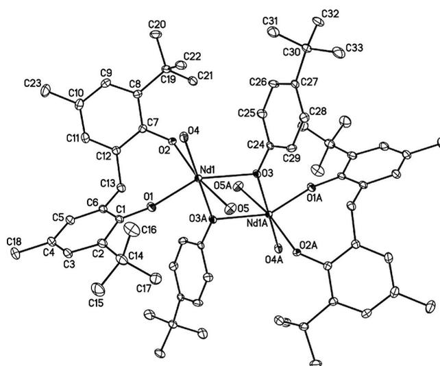
**Figure 3.** ORTEP diagram of complex **4** showing atom-numbering scheme. Thermal ellipsoids are drawn at the 20% probability level. Hydrogen atoms and carbon atoms on THF molecules are omitted for clarity.
