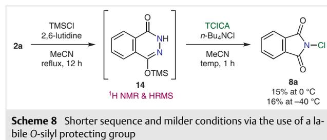
**Scheme 8** Shorter sequence and milder conditions via the use of a labile *O*-silyl protecting group
