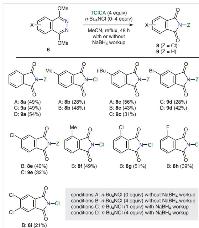
**Scheme 6** *N*-Chlorinative ring contraction of 1,4-dimethoxyphthalazines. The reactions were conducted with 1.0 mmol of **6** at 0.17 M concentration. Isolated yields after column chromatography are shown in the parenthesis. For **8i**: Reaction time: 5 days.
