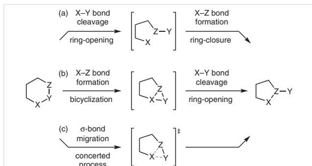
**Scheme 9** Three types of ring contraction mechanism: (a) ring-opening/ring-closure mechanism, (b) bicyclization/ring-opening mechanism, and (c) concerted  $\sigma$ -bond migration mechanism.
