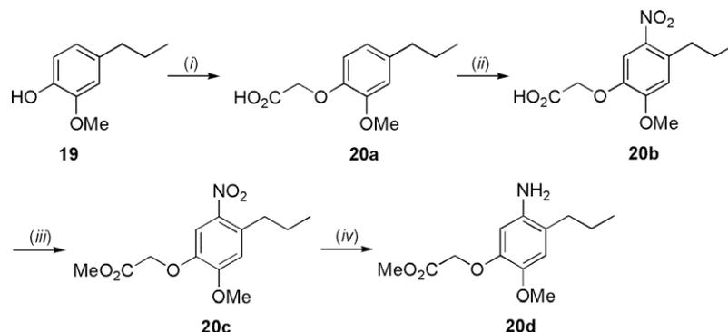
**Scheme 3.** Reagents and conditions: (i)  $\text{ClCH}_2\text{CO}_2\text{Na}$ , NaOH,  $\text{H}_2\text{O}$ ,  $60^\circ\text{C}$ , 24 h, 69%; (ii)  $\text{H}_2\text{SO}_4$ ,  $\text{HNO}_3$ ,  $20^\circ\text{C}$ , 24 h, 76%; (iii) MeOH, *p*-TsOH,  $60^\circ\text{C}$ , 2 h, 92%; (iv)  $\text{H}_2$  (30 psi), Pd/C, EtOAc,  $20^\circ\text{C}$ , 24 h, 80%.
