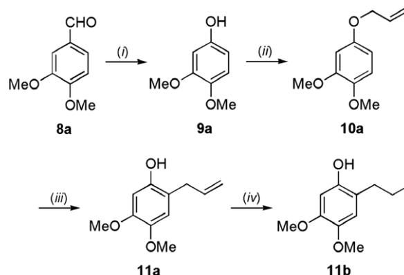
**Scheme 1.** Reagents and conditions: (i) (a) MCPBA, CH<sub>2</sub>Cl<sub>2</sub>, 20 °C, 6 h, 85%; (b) MeOH, HCl (6 N), 20 °C, 1 h, 89%; (ii) CH<sub>2</sub>=CHCH<sub>2</sub>Br, K<sub>2</sub>CO<sub>3</sub>, acetone, 60 °C, 6 h, 71%; (iii) decaline, 220 °C, 12 h, 86%; (iv) H<sub>2</sub>, Pd/C, EtOH, 20 °C, 12 h, 81%.
