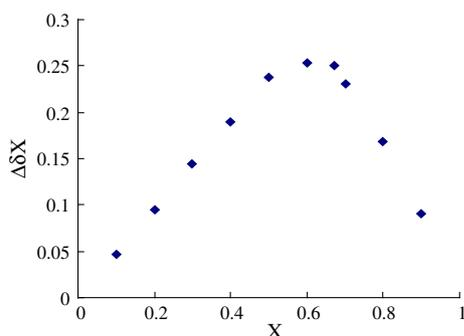
**Figure 7.** Job plots for the complexation of compound **1a** with **L-15**. ( $X = [\mathbf{1a}]/([\mathbf{1a}] + [\mathbf{L-15}])$ );  $\Delta\delta$  = variation of the chemical shift of the observed proton).
