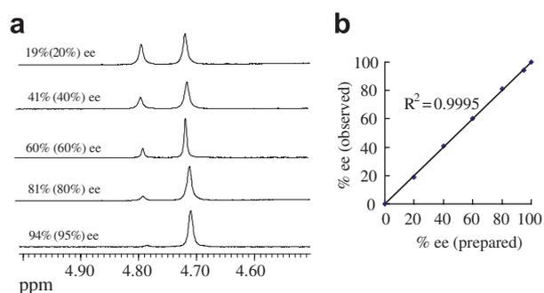
**Figure 8.** (a) Partial <sup>1</sup>H NMR (500 MHz) spectra of (*S*)-**4** with various enantiomeric purities (4 mM) in the presence of an equimolar amount of compound **1a**. (b) Correlation between the observed and prepared % ee values.
