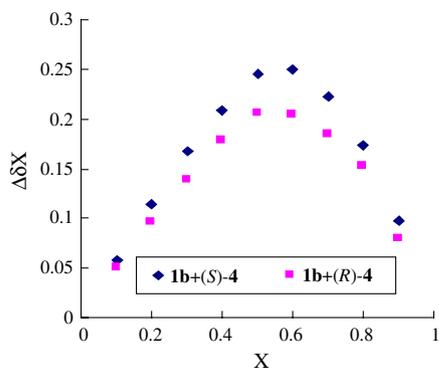
**Figure 6.** Job plots for the complexation of compound **1b** with (*R*)-**4** and (*S*)-**4**. ( $X = [\mathbf{1b}]/([\mathbf{1b}] + [\mathbf{4}])$ );  $\Delta\delta$  = variation of the chemical shift of the observed proton).
