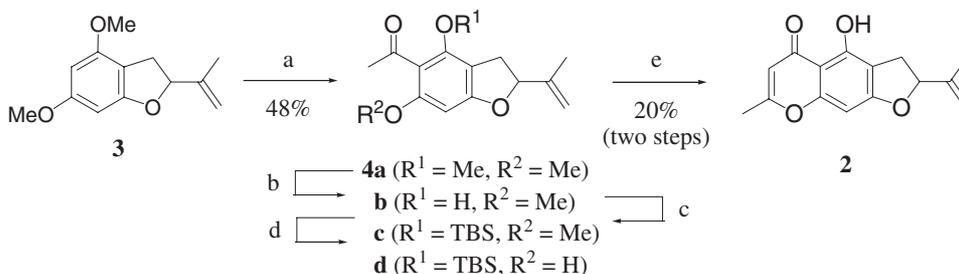
**Reaction conditions:** a)  $\text{CH}_3\text{CO}_2\text{H}$ ,  $(\text{CF}_3\text{CO})_2\text{O}$ , room temperature, 1 h; b)  $\text{MgI}_2\text{-OEt}_2$ , benzene, reflux, 3 h, 82%; c) TBSCl, NaH, THF, room temperature, 30 min, 83%; d)  $\text{MgI}_2\text{-OEt}_2$ , benzene, reflux, 15 h, 82%; e) 1)  $\text{CH}_3\text{C}(\text{OMe})_2\text{NMe}_2$ , xylene, reflux, 24 h; 2) 1 M TBAF, THF, room temperature, 1 h, 20% (two steps)
