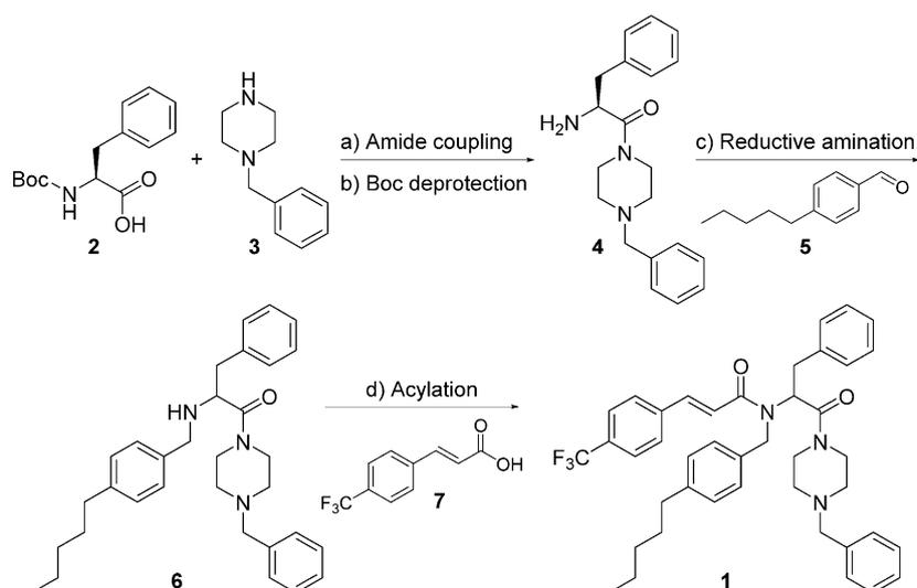
**Scheme 1.** Preparation of compound **1** as an illustration of the general synthetic pathway, showing readily accessible and efficient chemistry. (Further details are given in the Supporting Information).
