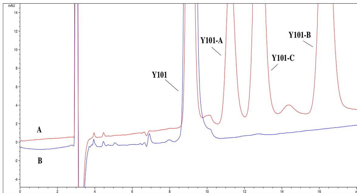
**Figure 4.** Expanded chiral HPLC chromatograms of **Y101**. A: a mixture of **Y101**, Stereoisomer **Y101-A** (2S, 2'R), Stereoisomer **Y101-B** (2R, 2'S) and Stereoisomer **Y101-C** (2R, 2'R); B: a crude reaction mixture of **Y101**.
