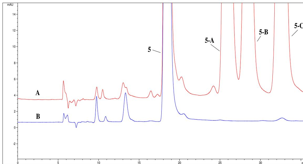
**Figure 3.** Expanded chiral HPLC chromatograms of intermediate **5**. A: a mixture of intermediate **5**, stereoisomer **5-A** (2S, 2'R), stereoisomer **5-B** (2R, 2'R) and stereoisomer **5-C** (2R, 2'S); B: a crude reaction mixture of intermediate **5**.
