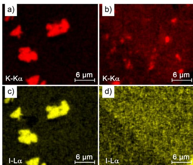
**Figure 5.** EDX element maps for K and I of (a,c) KI@poly18C6 and (b,d) KI@poly18C6 after run 10.
