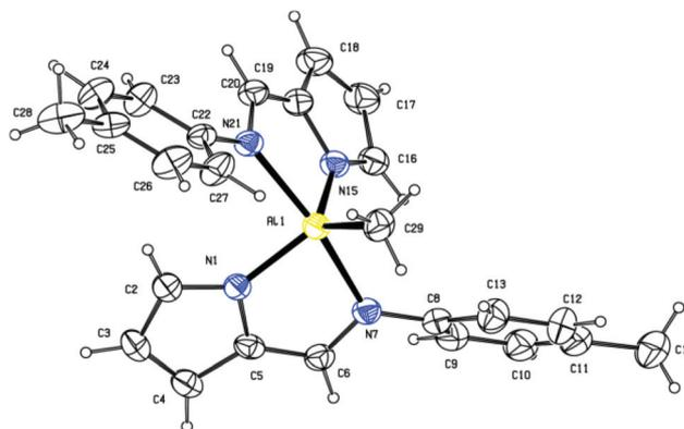
**Fig. 1** Molecular structure of  $L\frac{1}{2}AlMe$  (**1b**). Selected bond lengths (Å) and angles (°) are as follows: Al1–N21, 2.125(2); Al1–N7, 2.162(2); Al1–N1, 1.912(2); Al1–N5, 1.908(2); Al1–C29, 1.963(3); N1–Al1–N15, 115.47(9); N1–Al1–N21, 90.74(8); N1–Al1–N7, 80.23(8); N1–Al1–C29, 125.3(1); N15–Al1–N21, 81.38(9); N15–Al1–N7, 91.13(9); N15–Al1–C29, 119.3(1); N21–Al1–N7, 164.53(9); N21–Al1–C29, 97.9(1); N7–Al1–C29, 97.5(1).
