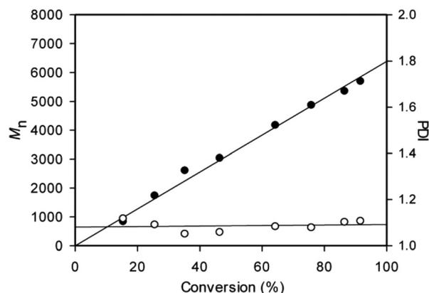
Fig. 2 Plots of PLA *M*<sub>n</sub> (●) and PDI (○) as a function of monomer conversion for a *rac*-LA polymerization using **1a**/PhCH<sub>2</sub>OH ([LA]<sub>0</sub>/[Al] = 50, toluene, 70 °C).
