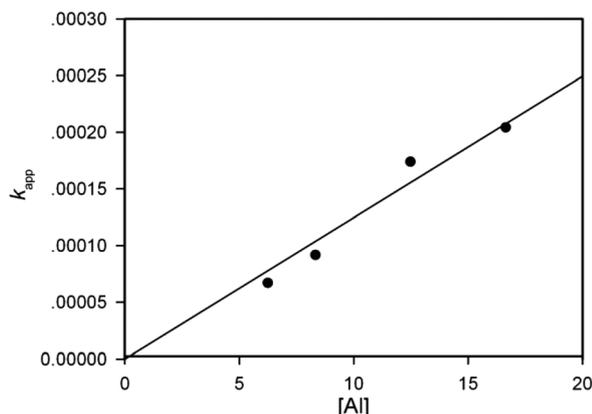
Fig. 6 Plot of  $k_{\text{app}}$  versus  $[\text{Al}]$  for the polymerization of *rac*-lactide with complex **1a**/ $\text{PhCH}_2\text{OH}$  as an initiator (toluene, 70 °C,  $[\text{LA}]_0 = 0.42 \text{ M}$ ).
