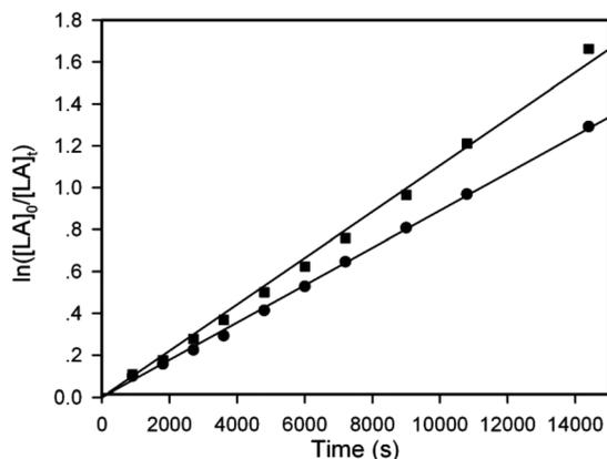
**Fig. 3** Semilogarithmic plots of *rac*-lactide conversion versus time in toluene at 70 °C with complexes **1a** (●) and **1b** (■) ([LA]<sub>0</sub>/[Al] = 50, [Al]/[PhCH<sub>2</sub>OH] = 1, [LA]<sub>0</sub> = 0.42 M, [Al] = 8.33 mM).
