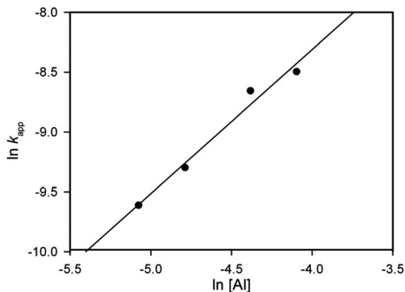
Fig. 5 Plot of  $\ln k_{\text{app}}$  versus  $\ln [\text{Al}]$  for the polymerization of *rac*-lactide with complex **1a**/ $\text{PhCH}_2\text{OH}$  as an initiator (toluene, 70 °C,  $[\text{LA}]_0 = 0.42 \text{ M}$ ).
