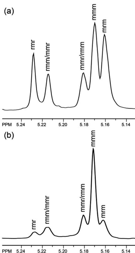
Fig. 7 Homonuclear decoupled <sup>1</sup>H NMR spectra of the methine region of PLA prepared from *rac*-lactide at 70 °C in toluene (500 MHz, CDCl<sub>3</sub>) with (a) **6b**/PhCH<sub>2</sub>OH and (b) **7b**/PhCH<sub>2</sub>OH.
