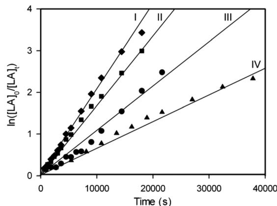
**Fig. 4** Semilogarithmic plots of the *rac*-lactide conversion versus time in toluene at 70 °C with complex **1a**/PhCH<sub>2</sub>OH as an initiator ([LA]<sub>0</sub> = 0.42 M: I, [Al] = 16.65 mM, [LA]<sub>0</sub>/[Al] = 25; II, [Al] = 12.49 mM, [LA]<sub>0</sub>/[Al] = 34; III, [Al] = 8.33 mM, [LA]<sub>0</sub>/[Al] = 50; IV, [Al] = 6.24 mM, [LA]<sub>0</sub>/[Al] = 67).
