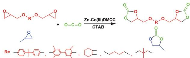
**Scheme 1** The one-pot coupling reaction of PO, bisepoxide and CO<sub>2</sub> catalyzed by the Zn–Co(III) DMCC/CTAB binary catalyst system.
