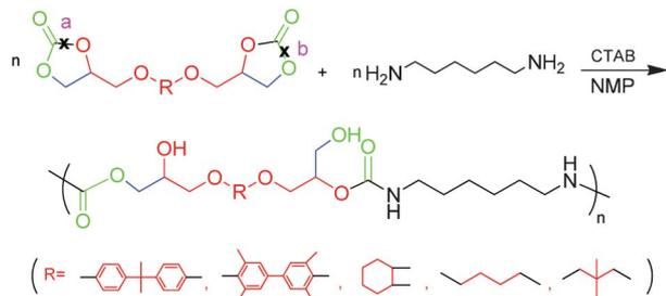
**Scheme 2** Polyaddition of bis(cyclic carbonate)s and 1,6-hexamethylenediamine. Note that two ways of ring opening of the carbonate via routes a and b occur randomly during reaction, leading to the formation of the secondary and primary hydroxyl groups.
