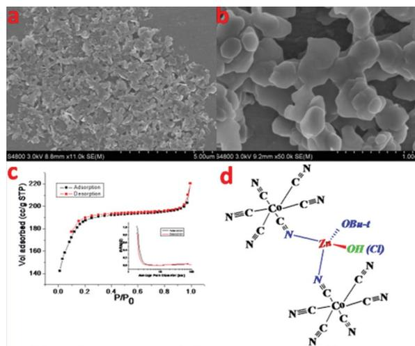
**Fig. 1** SEM images (a,b), nitrogen adsorption–desorption isotherm and pore size distribution (c) and the proposed local active site of the Zn–Co(III) DMCC catalyst (d).
