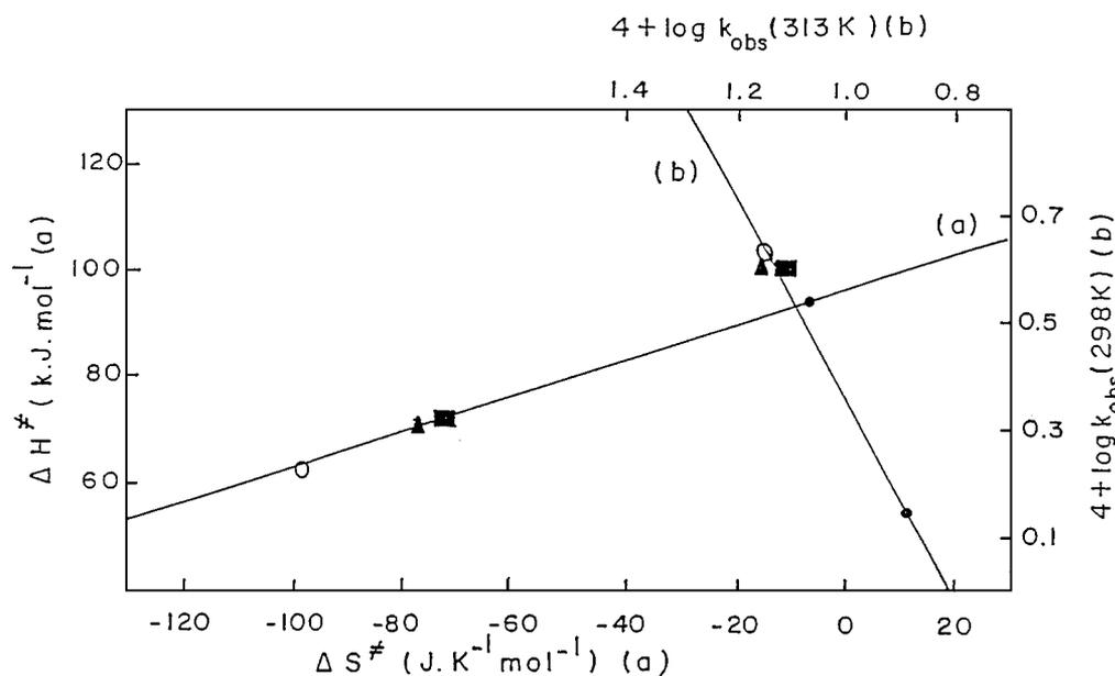
**FIGURE 2** Isokinetic plots of (a)  $\Delta H^\ddagger$  vs.  $\Delta S^\ddagger$  and (b)  $\log k_{\text{obs}}(313 \text{ K})$  vs.  $\log k_{\text{obs}}(298 \text{ K})$ :  $[\text{CAT}]_0 = 3.00 \times 10^{-3} \text{ mol dm}^{-3}$ ;  $[\text{amino acid}]_0 = 5.00 \times 10^{-2} \text{ mol dm}^{-3}$ ;  $[\text{HClO}_4] = 6.00 \times 10^{-2} \text{ mol dm}^{-3}$ .
