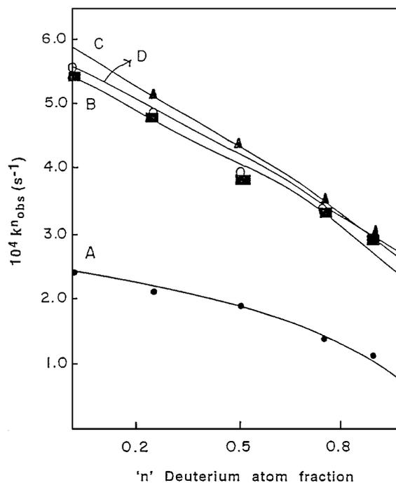
**Figure 1** Proton-inventory plots for the oxidation of  $\alpha$ -amino acids by CAT in  $H_2O$ – $D_2O$  mixtures at  $30^\circ C$ :  $[CAT]_0 = 3.00 \times 10^{-3} \text{ mol dm}^{-3}$ ;  $[\text{amino acid}]_0 = 5.00 \times 10^{-2} \text{ mol dm}^{-3}$ ;  $[HClO_4] = 6.00 \times 10^{-2} \text{ mol dm}^{-3}$ ; A: Gly; B: Val; C: Ala; D: Phe.
