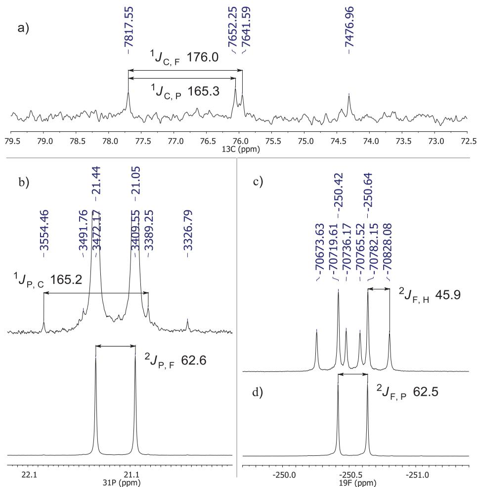
**FIGURE 2** Assignments of  ${}^1J_{C,P}$  and  ${}^1J_{C,F}$  in  ${}^{13}\text{C}$  NMR proton decoupled spectrum of **2d** (a) via the  ${}^{13}\text{C}$  satellites in  ${}^{31}\text{P}$  NMR proton decoupled spectrum (b);  ${}^{19}\text{F}$  NMR non-decoupled (c) and proton decoupled (d) spectra of **2d**. (Color figure available online).
