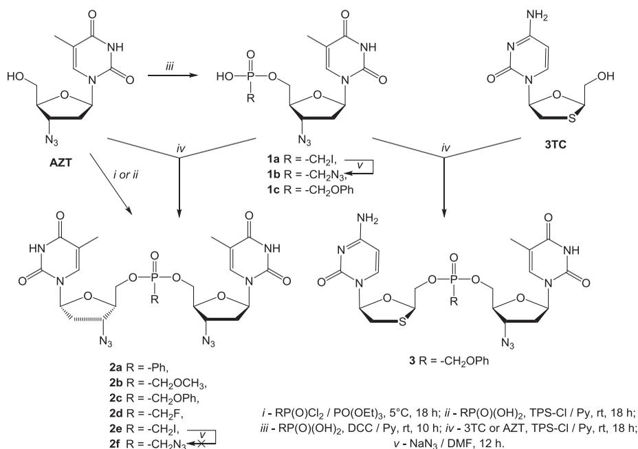
**SCHEME 1** Synthesis of homodimers of AZT (**2**) and a heterodimer of AZT and 3TC (**3**).
