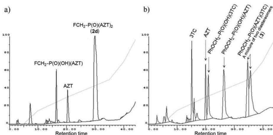
**FIGURE 3** HPLC separation of the hydrolysis products of **2d** and **3** after incubation with human blood serum. Products of compound **2d** after 50 min incubation (a); products of compound **3** after 12 hours incubation (b).
