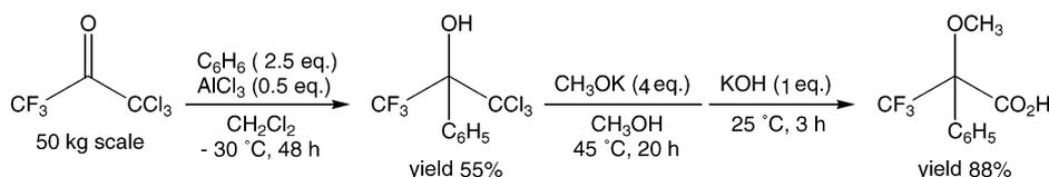
Scheme 4. Industrial synthetic method of Mosher's acid using TCTFA.
