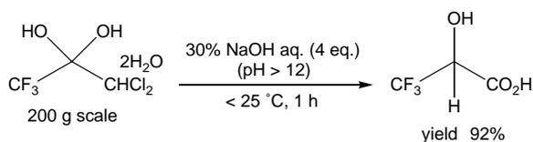
Scheme 2. Industrial synthetic method of trifluorolactic acid using DCTFA.
