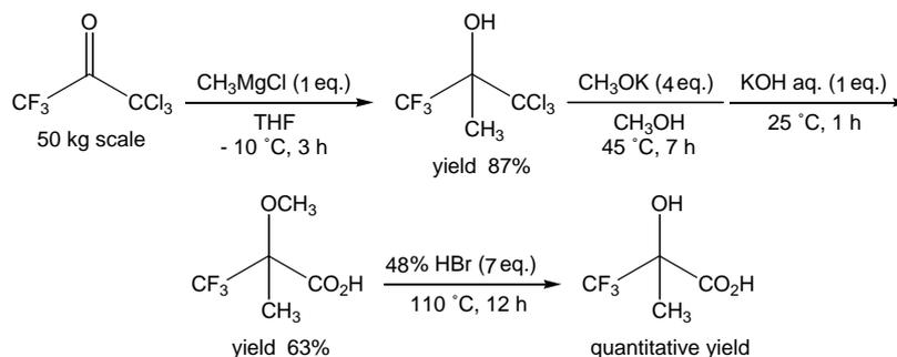
Scheme 3. Industrial synthetic method of  $\alpha$ -methyltrifluorolactic acid using TCTFA.
