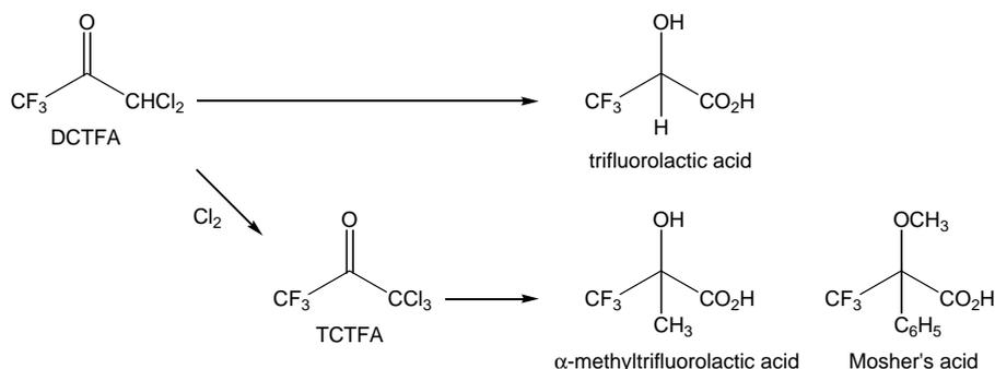
Scheme 1. Industrial synthetic methods of trifluorolactic acid derivatives using DCTFA and TCTFA.
