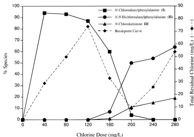
FIGURE 4. Product distribution in a wastewater (pH 7.0) inoculated with alanyl-*p*-[<sup>3</sup>H]-phenylalanine and chlorinated along the breakpoint curve (40–280 mg/L).
