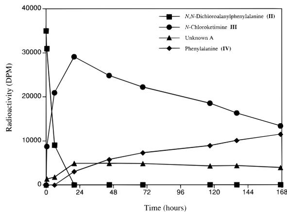
FIGURE 5. Product distribution in a wastewater (pH 7.0) inoculated with alanyl-*p*-[<sup>3</sup>H]-phenylalanine that was chlorinated to 240 mg/L and analyzed over 168 h.
