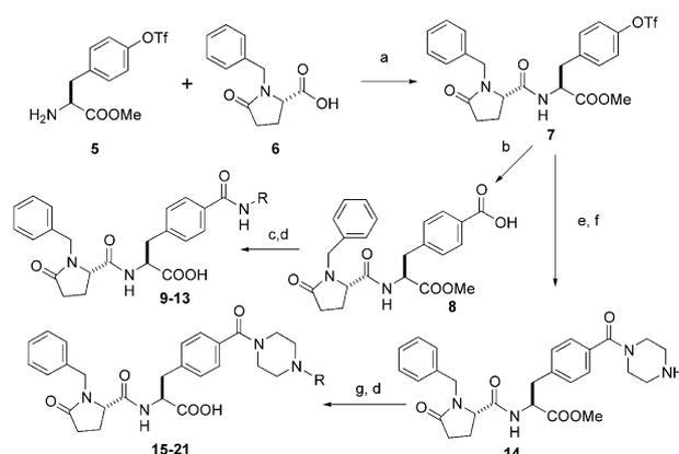
**Scheme 1.** Synthesis of 4-aminocarbonylphenylalanine analogues: (a) HBTU, DIEPA DMF, rt; (b) PdAc<sub>2</sub>, dppp, DMSO, CO, Et<sub>3</sub>N, H<sub>2</sub>O, 60 °C; (c) NH<sub>2</sub>R, HBTU, DIEPA, DMF, rt; (d) NaOH, EtOH, H<sub>2</sub>O, rt; (e) Pd(OAc)<sub>2</sub>, dppp, *N*-Boopiperazine CO, Et<sub>3</sub>N, 60 °C; (f) 4 N HCl in cloxane; (g) benzoic acids, HBTU, DIPEA, rt; or benzenesulfonyl chloride, DCM, DIPEA, rt.
