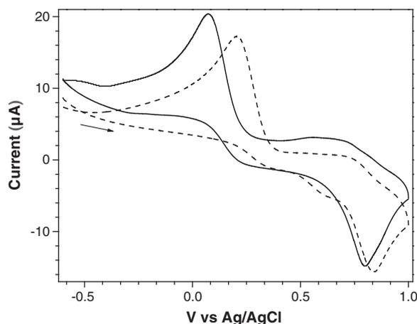
Fig. 2. Cyclic voltammograms of a  $10^{-3}\text{ M}$  solution of **1** (solid) and **2** (dotted) in dichloromethane in presence of  $0.1\text{ M}$  TBAP as a supporting electrolyte, glassy-carbon as a working electrode; scan rate  $0.1\text{ V/s}$ .
