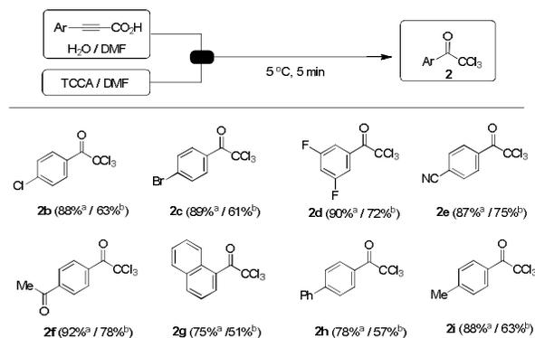
**Scheme 1.** Synthesis of 2,2,2-trichloroacetophenone derivatives using a flow reaction system. Reaction condition: Reservoir A = **1** (4.25 mmol) / H<sub>2</sub>O (68.0 mmol) / DMF (15.0 mL), Reservoir B = TCCA (4.25 mmol) / CH<sub>3</sub>CN (15.0 mL) <sup>a</sup>Isolated yield. <sup>b</sup>Yield from the batch reaction. Reaction condition : **1** (2.0 mmol), TCCA (2.2 mmol) and H<sub>2</sub>O (32.0 mmol), were reacted in CH<sub>3</sub>CN (5.0 mL) at 25 °C for 12 h.
