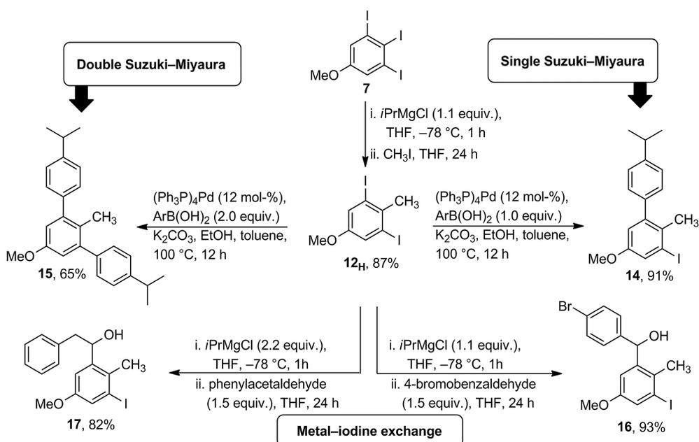
Scheme 4. Possible chemical transformations toward disubstituted and trisubstituted anisole derivatives from 3,4,5-triiodoanisole (**7**).
