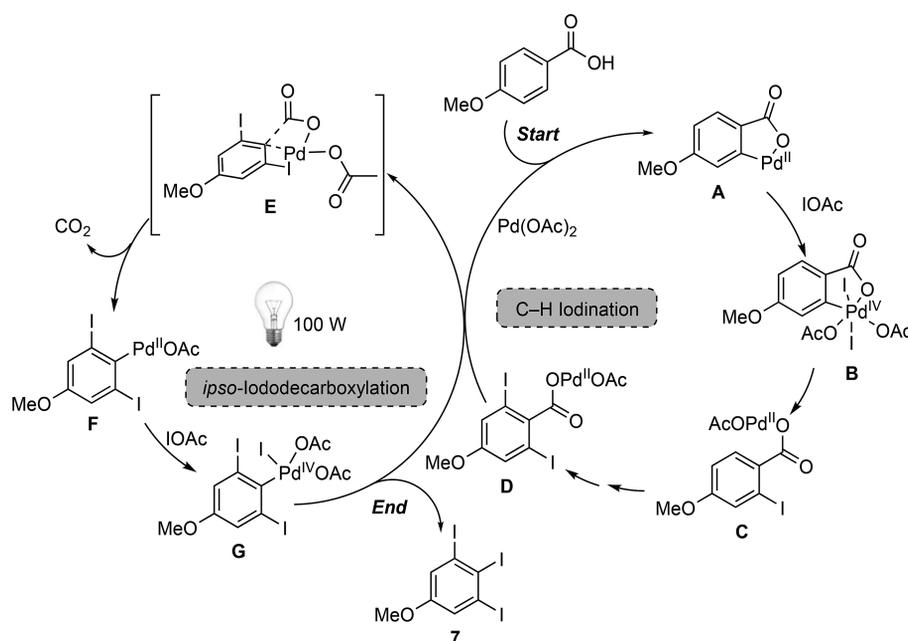
Scheme 2. Proposed mechanism for the one-pot  $\text{Pd}^{\text{II}}$ -catalyzed C–H iodination/*ipso*-iododecarboxylation of *para*-anisic acid.
