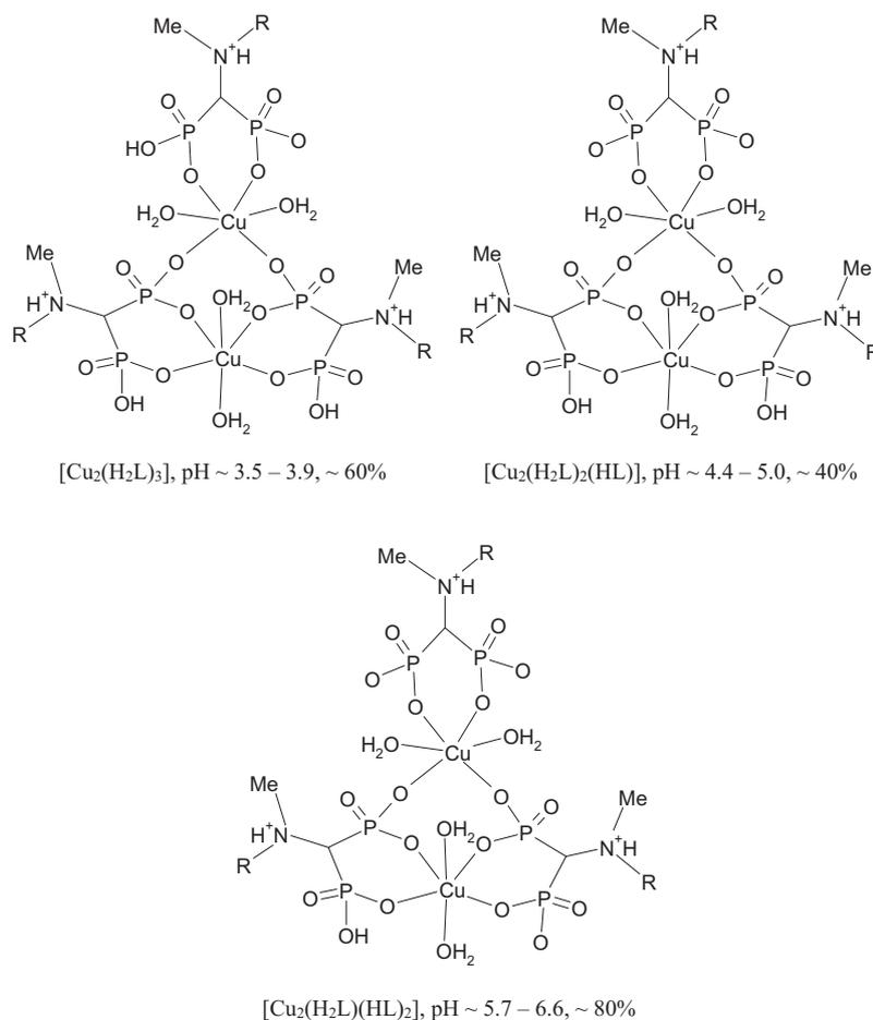
**Scheme 6.** Schematic representations showing the possible structures of the dinuclear complex species formed in the in the water solution of Cu(II)–L systems and pH range of their maximum concentration.
