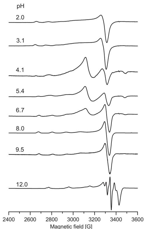
**Fig. 4.** The EPR spectra due to an aqueous solution containing Cu(II) ions and ligand **3a** depending on pH at 77 K for 1:3 metal-to-ligand molar ratios;  $C_{\text{Cu(II)}} = 4 \times 10^{-3}$  M.
