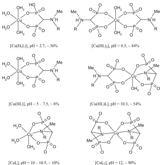
**Scheme 5.** Schematic representations showing the possible structures of the mononuclear complex species formed in the water solution of Cu(II)–L systems and pH range of their major concentration.
