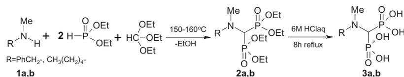
**Scheme 2.** Direct synthesis of *N*-methyl alkylaminomethane-1,1-diphosphonic acids **3a** and **3b**.
