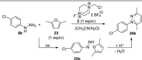
**Scheme 7.** Trapping of the phenyldiazene intermediate **22b** by cycloaddition to 2,5-dimethylfuran (**23**).
