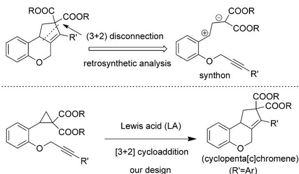
Scheme 1. Design of a Lewis acid-catalyzed ring expansion of cyclopropane 1,1-diester.
