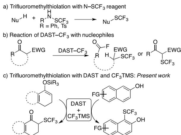
**Scheme 1.** DAST &  $\text{CF}_3\text{TMS}$  as electrophilic trifluoromethylthiolating reagent with 'C'-nucleophile.
