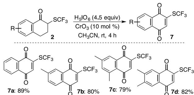
**Scheme 5.** Synthesis of  $\alpha$ -trifluoromethylthiolated naphthoquinone **7**.
