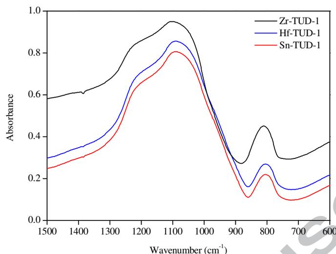
**Figure 4.** Skeletal FT-IR spectra of Zr-, Hf- and Sn-TUD-1.
