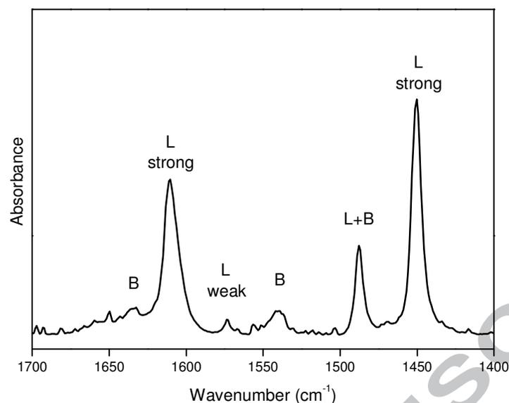
**Figure 5.** FT-IR spectrum of pyridine adsorbed at 150 °C on Sn-TUD-1. Signals attributed to pyridine adsorbed on Brønsted acid sites are labelled with B and on Lewis acid sites with L.
