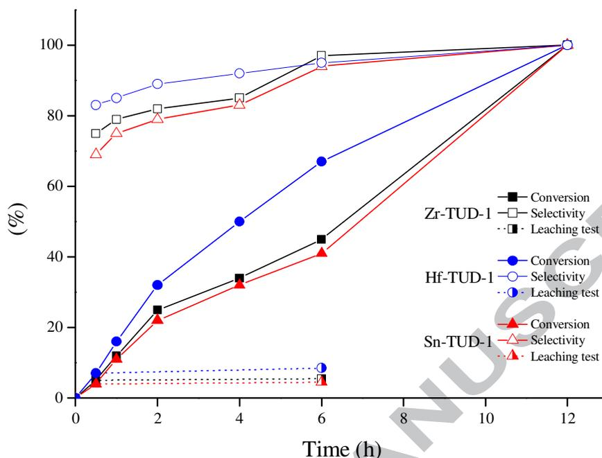
**Figure 6.** Kinetic study on the conversion of dihydroxyacetone over metal-containing TUD-1 catalysts. Reaction conditions: 5 ml of 0.4 M DHA, 100 mg of catalysts, 90°C. Leaching test results are presented with half-filled symbols.
