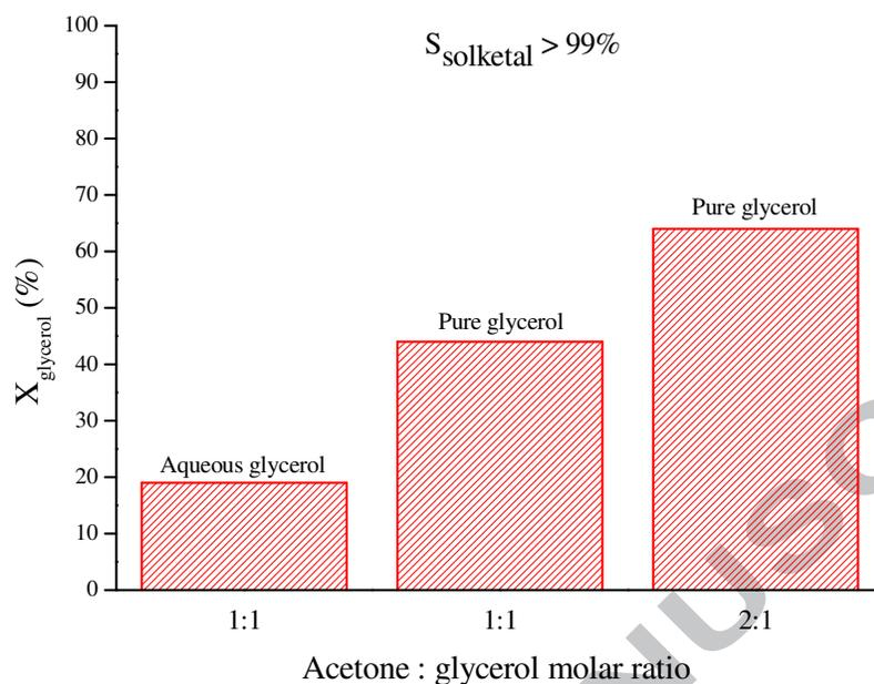
**Figure 8.** Conversion of glycerol in the synthesis of solketal catalysed by Sn-TUD-1. Reaction conditions:  $1.00 \cdot 10^{-2}$  mol glycerol,  $1.00 \cdot 10^{-2}$  mol acetone ( $2.00 \cdot 10^{-2}$  mol acetone in the last test), *tert*-butanol ( $1.00 \cdot 10^{-2}$  mol) as solvent, 25 mg of catalyst, 80 °C, 6h.
