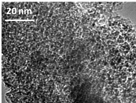
**Figure 2.** TEM image of Sn-TUD-1. The corresponding images for Zr- and Hf-TUD-1 can be found in ref. [36].
