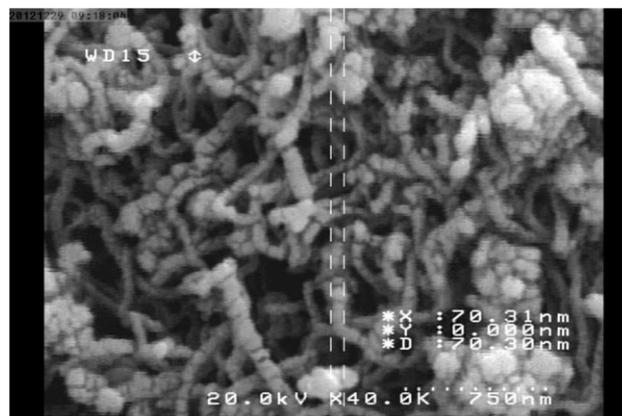
**Figure 2.** Scanning electron microscope image of magnetic nanocomposite of multiwalled carbon nanotube. [Color figure can be viewed at [wileyonlinelibrary.com](http://wileyonlinelibrary.com)]
