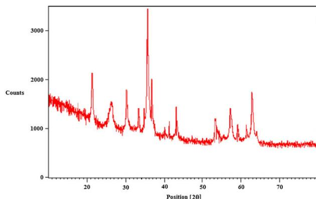
**Figure 1.** X-ray diffractometer pattern of magnetic nanocomposite of multiwalled carbon nanotube. [Color figure can be viewed at [wileyonlinelibrary.com](http://wileyonlinelibrary.com)]
