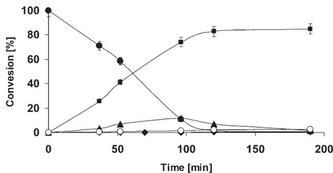
**Figure 4.** Reaction course of the conversion of cephalosporin C into 7-aminocephalosporanic acid using the trienzymatic, one-pot process. The reaction was carried out as described in the Experimental Section; ■: 7-ACA. ●: CPC. ▲:  $\alpha$ -ketoamidopyl-7-ACA; ○: side products and ◆: GL-7-ACA.
