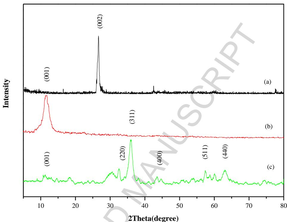
**Fig. 1** XRD pattern of graphite (a), GO (b), and Fe<sub>3</sub>O<sub>4</sub>/GO-Mo (c)
