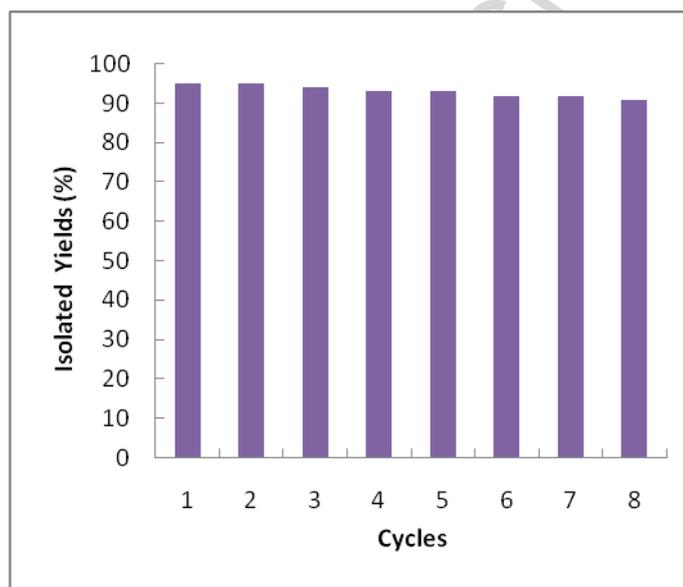
**Fig. 4** Reusability of the  $\text{Fe}_3\text{O}_4/\text{GO-Mo}$  in ChCl/urea catalytic system in the model reaction. Reaction conditions: isatin (10 mmol), malononitrile (10 mmol), and 4-(*p*-tolylamino)furan-2(5*H*)-one (10 mmol), catalyst (200 mg) in ChCl/urea (10 ml).
