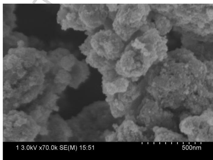
**Fig. 3** SEM image of  $\text{Fe}_3\text{O}_4/\text{GO-Mo}$ .
