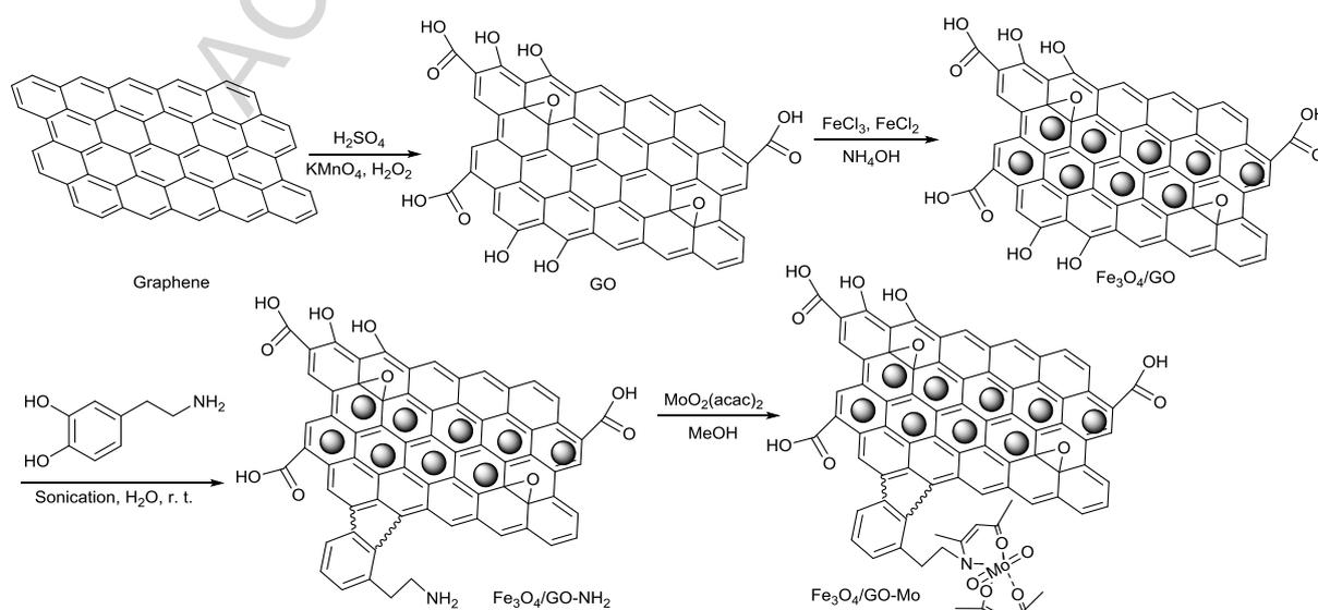
**Scheme 1** Preparation of Fe<sub>3</sub>O<sub>4</sub>/GO-Mo
