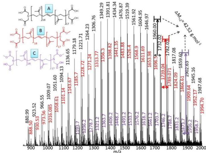
**Figure 1.** Electrospray ionization mass spectrum of IDA-PMO<sub>x33</sub>-IDA after alkaline hydrolysis at 50 °C for 16 h in the presence of 0.025 M NaOH solution.
