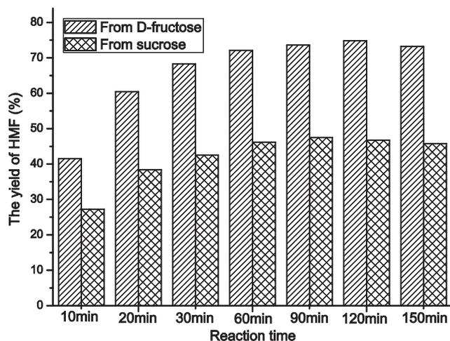
**Figure 2.** Effect of reaction time on the dehydration of D-fructose and sucrose.
