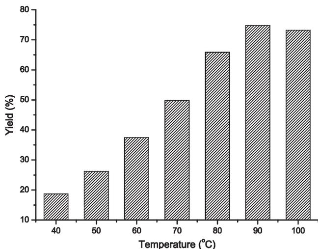
**Figure 1.** Effect of temperature on the dehydration of D-fructose.
