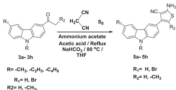
on further reaction with two equivalents of elemental sulfur in THF solvent and  $NaHCO_3$  as a base catalyst, resulted in the formation of bis-thiophene, that is, 4,4''-(9-ethyl-9*H*-carbazole-3,6-diyl)bis(2-minothiophene-3-carbonitrile) **17** in good yield (Table 3) (Scheme 5).
