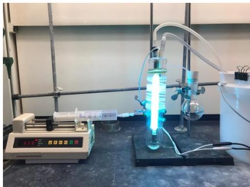
**Figure 2.** Flow photochemistry setup with syringe pump
